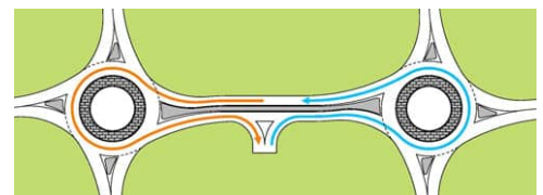
Tandem roundabouts with a continuous raised median eliminates left-turn and across-roadway conflicts. Source: FHWA
